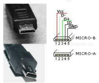
Micro-USB is a standard USB connector for a wide range of portable devices, including cell phones and smartphones
