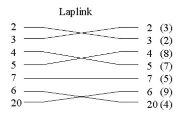
Numbers in brackets apply to 9 pin ports.
