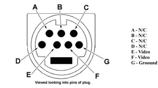
For Video out from a Video card using a 7 pin mini-din connector
